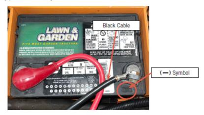
5. Using the appropriate tools, remove the retaining nut and bolt and keep for installation
